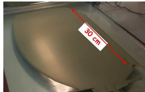
Figure 2: Tape casted and dried.
